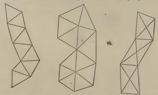
triangulation and the topography of the country will determine the location of the stations and the size of the triangles. A chain net is one suitable for a river survey, a polygonal net where the triangles from one or more polygons is some-
